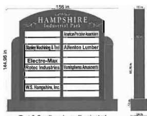
Text & Scroll work are illuminated Sign designed for 20 slots
